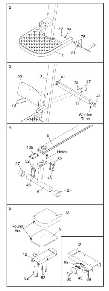
6. Pull the Seat Knob (45, not shown) out as far as it will go, and slide the Seat Carriage (12) onto the Bench Rail (5). Engage the Seat Knob into the third hole from the end of the Bench Rail.
